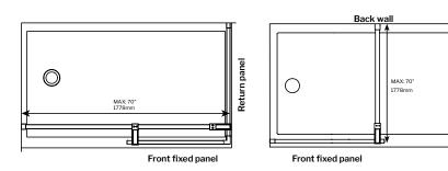
Support bar can be installed from wall to return panel, or from back wall to front fixed panel, up to a maximum of 70" length. For installation manual, see www.fleurco.com
