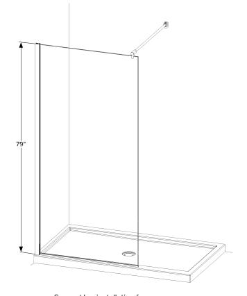
Support bar installation from back wall to fixed panel
